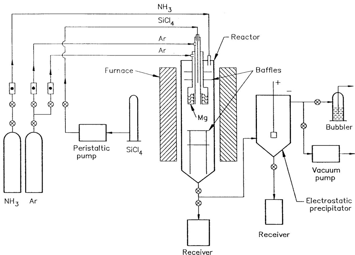
Figure 2 Schematic flow diagram of experimental apparatus for synthesis of silicon powder.
