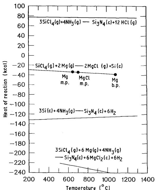
Figure 1 Heat of reaction for the reactions of  $\text{SiCl}_4$  and  $\text{NH}_3$ ,  $\text{SiCl}_4$  and magnesium, silicon and  $\text{NH}_3$ , and  $\text{SiCl}_4$ , magnesium and  $\text{NH}_3$ .
