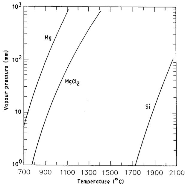
Figure 3 Vapour pressures of magnesium,  $\text{MgCl}_2$  and silicon pertinent to vacuum distillation. Melting temperature Mg = 651 °C;  $\text{MgCl}_2$  = 712 °C; Si = 1420 °C.
