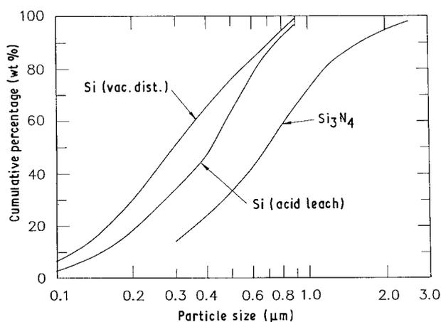
Figure 5 Particle-size distributions of vacuum-distilled and acid-leached silicon powders and  $\text{Si}_3\text{N}_4$  powder.
