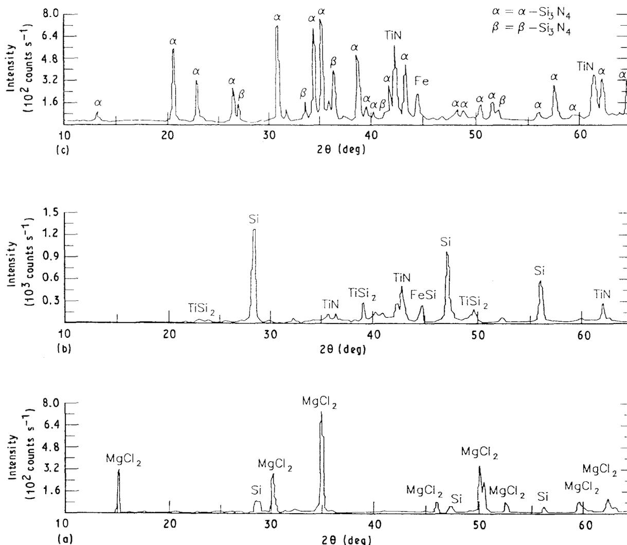
Figure 4 X-ray diffraction patterns of (a) powder obtained from reaction of SiCl<sub>4</sub> and magnesium at 1050 °C, (b) vacuum-distilled powder at 880 °C, and (c) nitrided silicon powder at 1150 °C.
